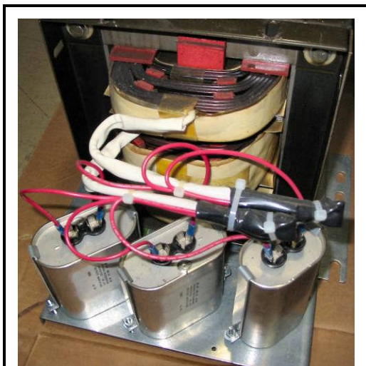
Ferroresonant transformer with capacitors for tuning circuit
